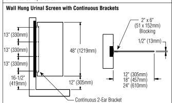
Generally used where specifications require the Urinal Screen to have a continuous bracket.
