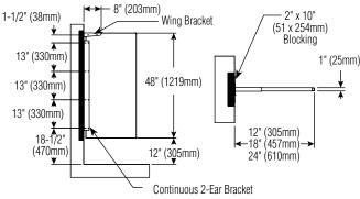
Generally used where specifications require the Urinal Screen to have a continuous bracket in addition to the Mills wing bracket.
