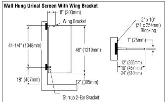
Generally used for Urinal Screen application where added durability is needed for high traffic areas. Screen is mounted to wall with Mills stainless steel wing bracket and 2-ear stirrup bracket.
